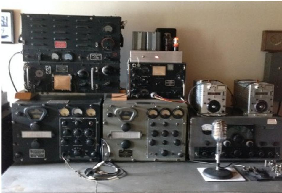
The Navy RBC-1 receiver is the gray receiver on the desk, while the TCS-13 Navy transmitter with HB Power Supply is atop the RBC.
