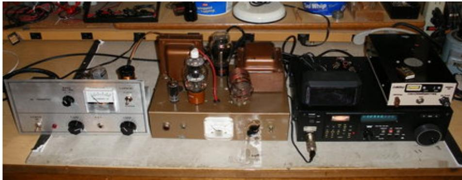
Kelvin 150-03: This one was an eBay find....a kit in its unopened box. Sure enough, it was indeed a kit in the true meaning of the word. All holes in the panel and chassis had to be drilled, punched, etc. No Heathkit style wiring instructions.....just a schematic, wiring pictorials and a few notes.
