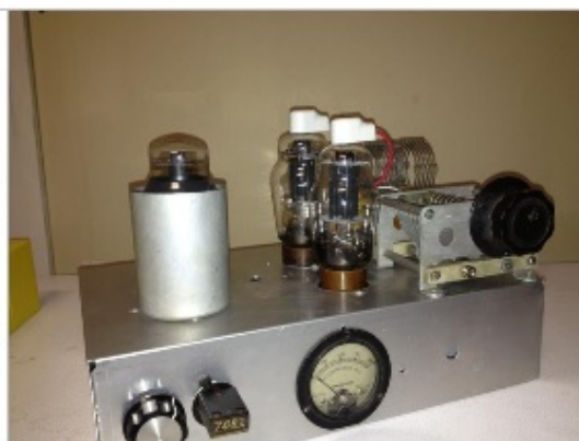
HB 807s driven by a 42 tube
