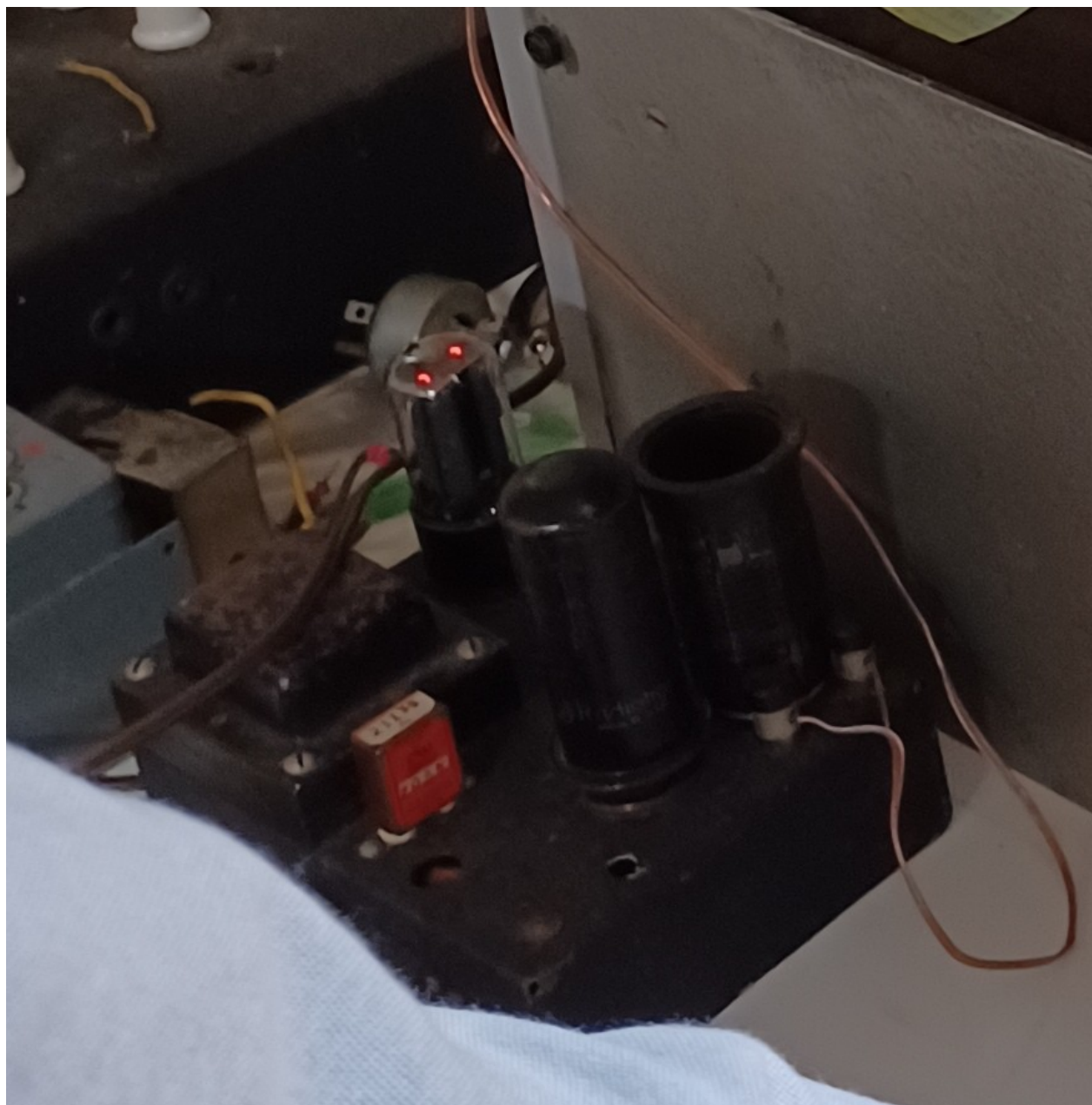
Close up of the outboard 3 Watt crystal 6L6 Driver.
